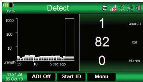
The display provides a historical graph of the intensity of the source. To the right of the history the real-time count rate and dose rate are shown constantly on every screen providing the much needed info to the user at all times.
