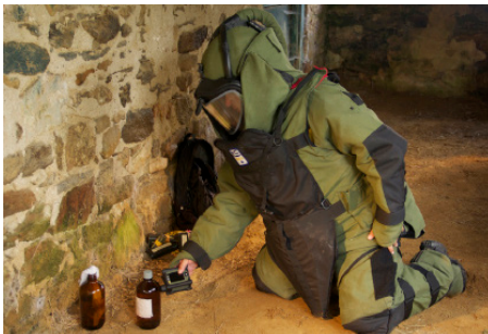
Fast and easy analysis of multi-layered liquids, no sampling required.
